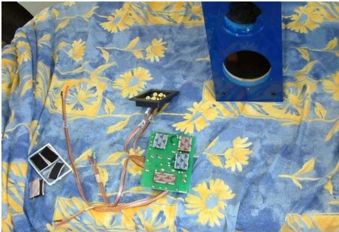
Fit crossover assembly through lower woofer hole and secure with the Velcro tabs onto the felt at bottom of speaker box
